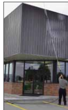
Telescoping wands extend to 24-ft. to reach high places without scaffolding
